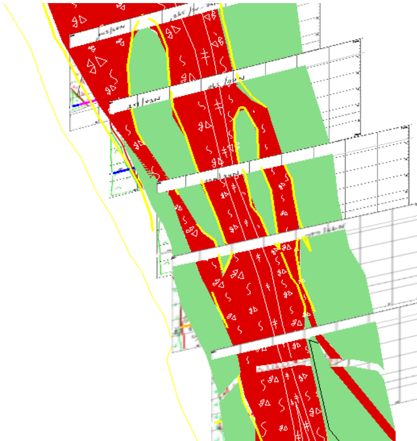
Figure 1. Slight oblique plan view of back-mapping of a level. Green is andesite country rock; red is vein material; bold yellow is a surveyed line of the vein contacts; fine yellow is the floor string of the drive.
